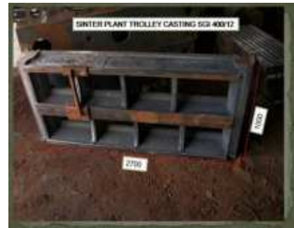
SINTER PLANT TOLLEY CASTING SGI
